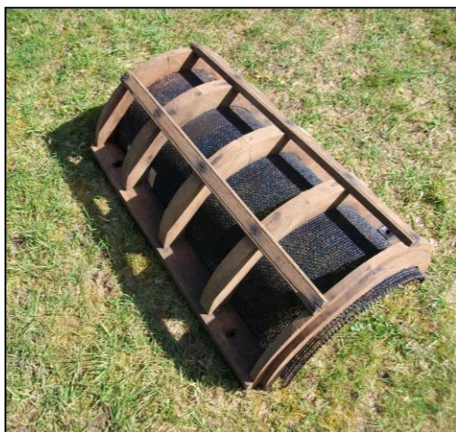
The picture left shows half of the smutter drum after preservation, with five elm rings supporting the coarse mesh lining.
