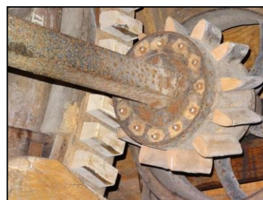
Skew gear and transverse layshaft driving additional machines at Jill
