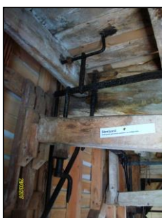
Part of the tentering gear of the tail stones is shown left, with the brayer end and adjusting screw visible. This is attached to the end of the steelyard, which is suspended on a nearby loop, creating a lever with a large mechanical advantage to support the weight of the runner stone.
