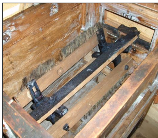
The picture left shows half of the smutter drum after preservation, with five elm rings supporting the coarse mesh lining.
