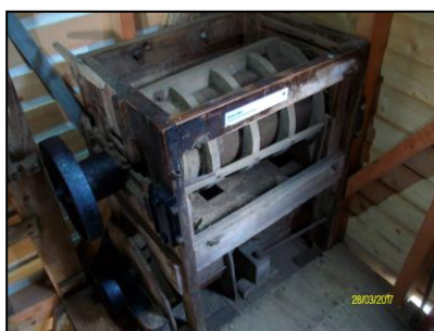
Smutter showing belt drives, drum and fan below
