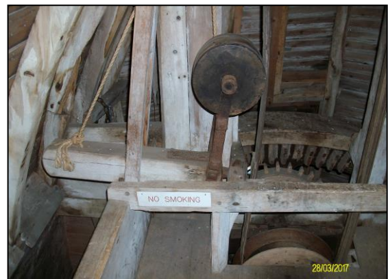
The picture above shows the sack hoist mechanism with the jockey wheel, crank and rope on the left, and the top of the brake wheel, drive gear, pulley and belt on the right.
